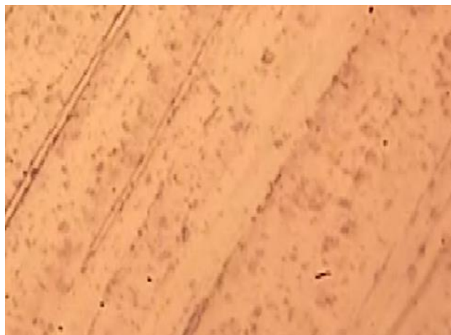
Fig. 4. Microstructure of commercially pure titanium (C.P.Ti) without adding carbon (X1000).
