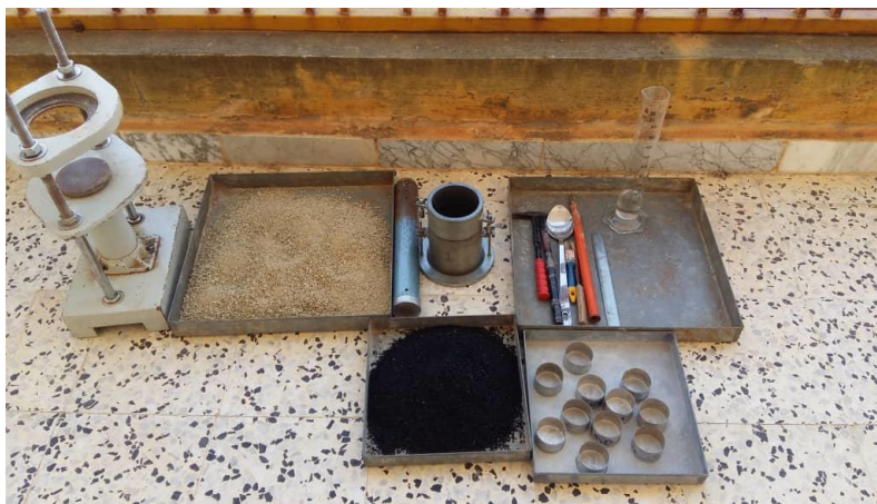
Fig. 5. The Compaction test.
