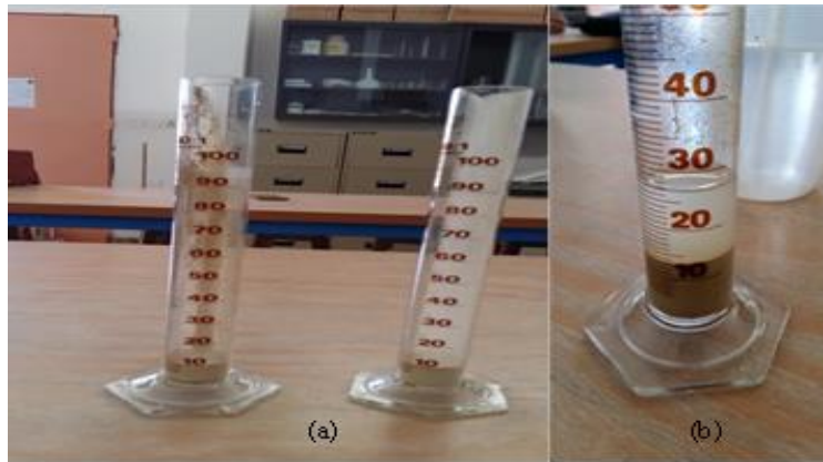
Fig. 4. The free swell of soil (a) and (b).
