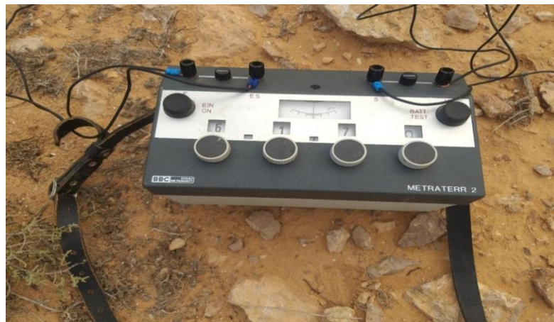
Figure 9: Soil resistivity meter
